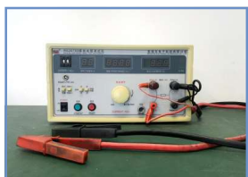
Ground Resistance Test
